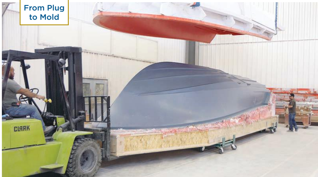
From Mold to Hull
